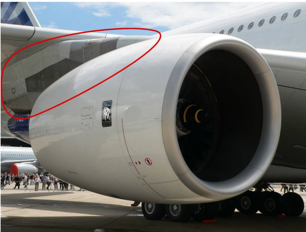
Figure 4: An Airbus A380’s engine pylon (thanks to Wikimedia Commons user David.Monniaux for the photo)
