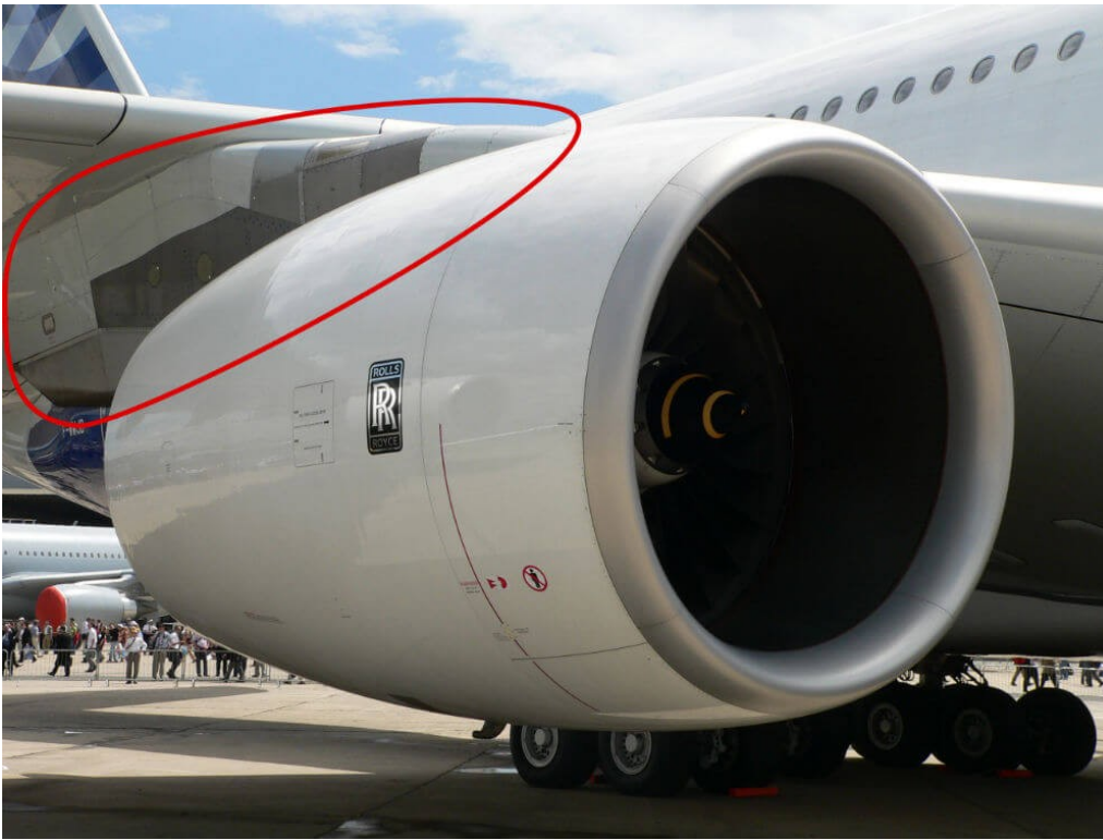
Figure 3.40: An Airbus A380's engine pylon (thanks to Wikimedia Commons user David.Monniaux for the photo)
