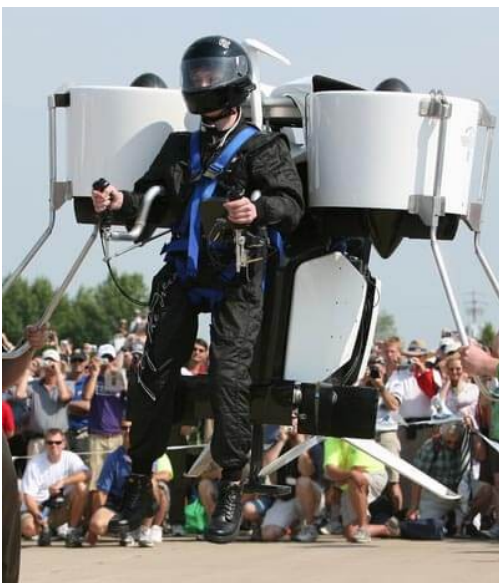
Figure 4.8: The Martin Jetpack, with its ducted fans (thanks to Flickr user martinjetpack for the photo)
