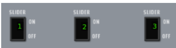
Figure 5.2: Three sliders in an instrument panel, whose numbers are displayed by pressing the Alt (Option) key
